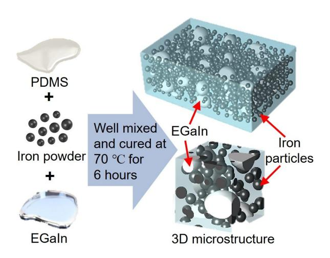
Schematic of the procedure for fabricating the liquid metal-filled magnetorheological elastomer Credit: Yun et al
