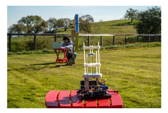
A new compact antenna for very low frequency (VLF) transmissions, developed and tested at SLAC, consists of a 4-inch-long piezoelectric crystal (clear rod at center) that generates VLF radiation. Credit: Dawn Harmer/SLAC National Accelerator Laboratory
