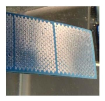
Complex biomimetic structures retain air under water. The air on the actually blue carrier appears silvery under water. Credit: Thomas Schimmel, KIT
