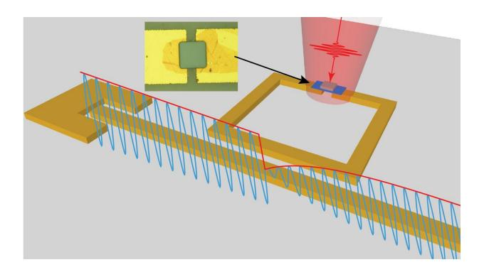
Rendering of the microwave resonator showing the (blue) microwave signal's size change resulting from a light pulse (red) once the pulse hits the infrared pixel (micrograph image of pixel is shown in the inset). Credit: Cockrell School of Engineering, The University of Texas at Austin
