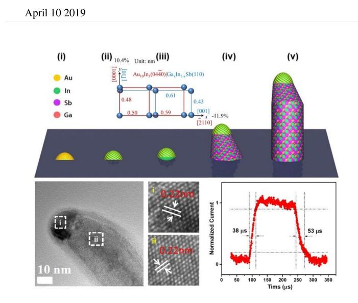
The growth mechanism and fast 1550 nm IR detection of the single-crystalline In0.28Ga0.72Sb ternary nanowires Credit: HAN Ning
