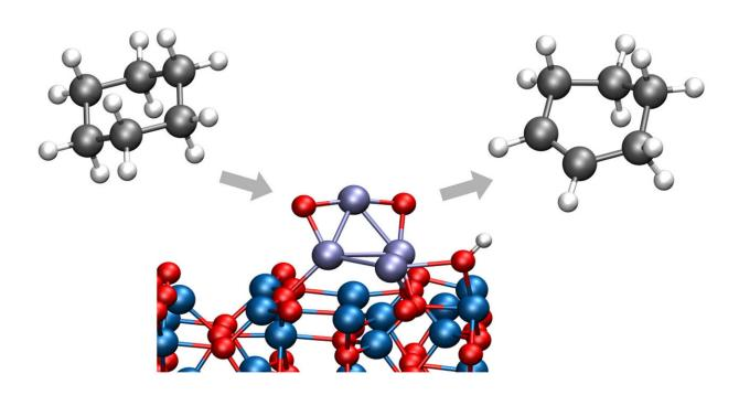
Argonne chemists have identified a way to convert cyclohexane to cyclohexene or cyclohexadiene, both important chemicals in a wide range of industrial processes. The new process takes place at low temperatures, eliminating the creation of unwanted byproducts. Credit: Argonne National Laboratory
