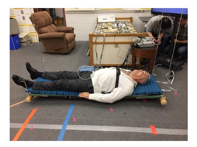
Ten years ago, Skubic's team developed hydraulic sensors that can be placed under a bed mattress to measure a person's heart rate and respiration rate. The team used those sensors on this hanging bed to gather data for the mathematical model used in this study. Credit: University of Missouri
