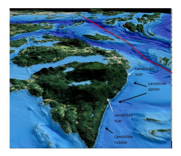
Image showing landslide failures around Orcas Island. The red line marks the newly discovered Skipjack fault zone. Credit: H. Gary Greene
