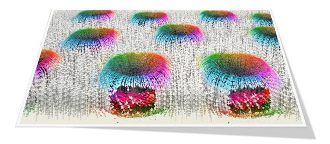
Army-funded research discovery may allow for development of novel device structures that can be used to improve logic/memory, sensing, communications, and other applications for the Army as well as industry. Image demonstrates simulation of emergent chirality in polar skyrmions for the first time in oxide superlattices. Credit: Xiaoxing Cheng, Pennsylvania State University; C.T. Nelson, Oak Ridge National Laboratory; and Ramamoorthy Ramesh, University of California, Berkeley
