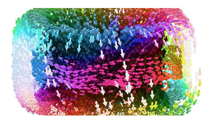
Simulation of a single polar skyrmion. Red arrows signify that this is a left-handed skyrmion. The other arrows represent the angular distribution of the dipoles. Credit: Xiaoxing Cheng, Pennsylvania State University; C.T. Nelson, Oak Ridge National Laboratory; and Ramamoorthy Ramesh, Berkeley Lab
