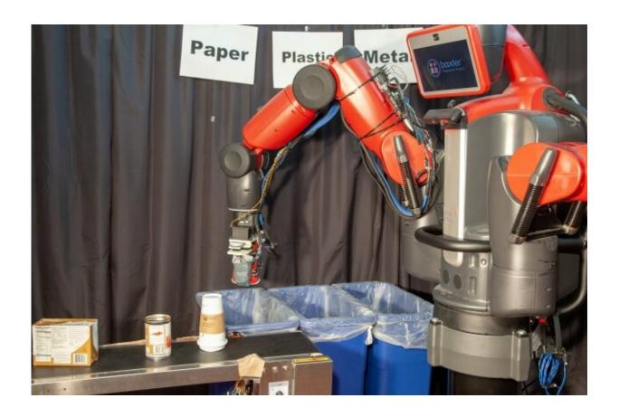
RoCycle can detect if an object is paper, metal, or plastic. CSAIL researchers say that such a system could potentially help enable the convenience of single-stream recycling with lower contamination rates that confirm to China's new recycling standards. Credit: Jason Dorfman
