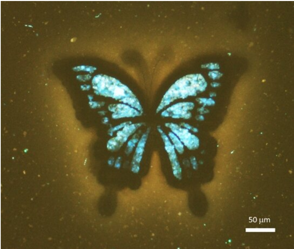
Figure shows a multicolour butterfly design which is made by patterning recovered carbon black in ambient and helium environments. Credit: National University of Singapore
