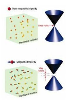
Top: Topological insulator doped with TR-invariant impurities with Dirac point similar to in undoped case. Bottom: Topological insulator doped with TR-breaking impurities with broken Dirac point. Credit: FLEET
