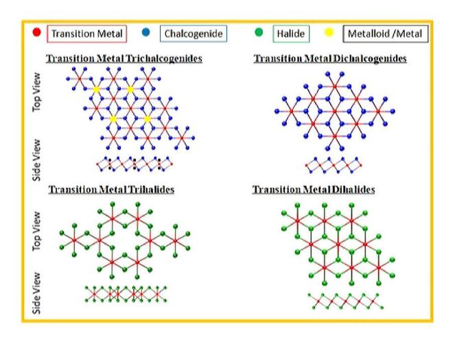
Crystal structures of proposed 2D ferromagnetic materials. Credit: FLEET
