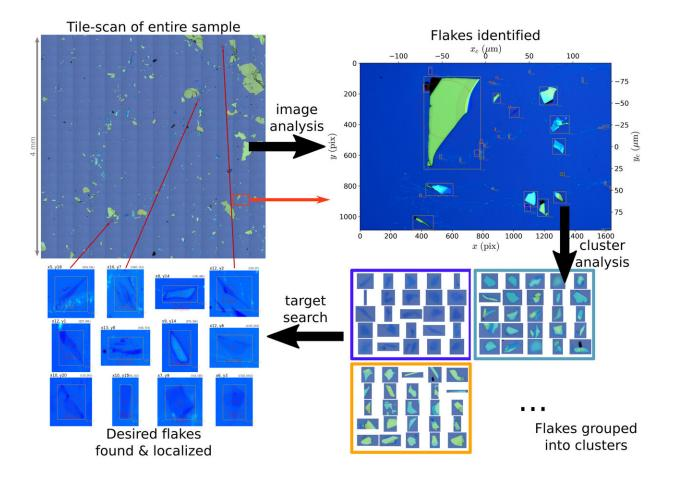
A schematic showing the workflow for cataloging flake locations and properties. Image grids of exfoliated samples are automatically analyzed, with each flake tracked individually so that scientists can locate any desired flake on a sample. Credit: Brookhaven National Laboratory
