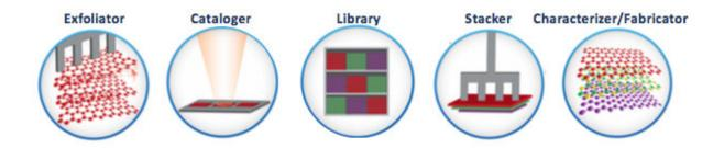
The QPress will have five modules when completed: an exfoliator, a cataloger, a materials library, a stacker, and a characterizer/fabricator. Credit: Brookhaven National Laboratory
