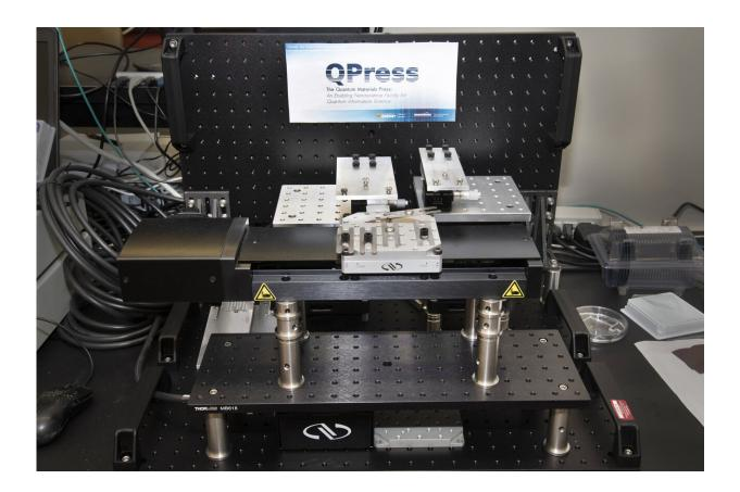
A photo of the prototype exfoliator. The robotic system transfers peeled 2-D flakes from the parent crystal to a substrate. The exfoliator allows scientists to control stamping pressure, pressing time, number of repeated presses, angle of pressing, and lateral force applied during transfer, for improved repeatability. Credit: Brookhaven National Laboratory
