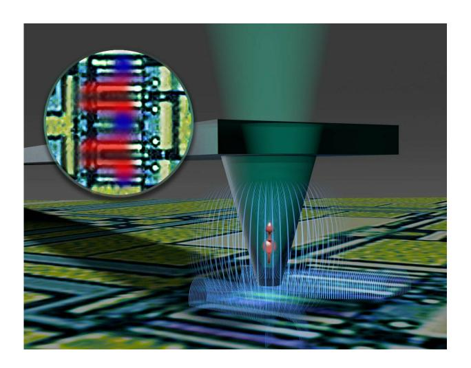
Schematic visualization of a scanning probe quantum magnetometer with an NV diamond tip that can detect and visualize currents in nanoelectronic circuits. Credit: Fraunhofer IAF
