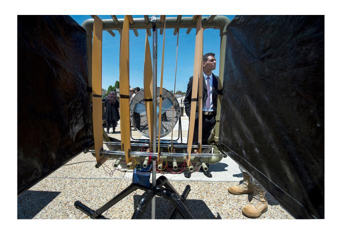
Axy Pagan-Vasquez, a mechanical engineer with the U.S. Army Corps of Engineers, explains how low-velocity wind energy is being captured using flexible strips of material during the Department of Defense Lab Day at the Pentagon. The US Army Corps of Engineers' Engineer Research and Development Center is developing the technology for use in conditions beyond suitable for wind turbines. Credit: EJ Hersom/DoD
