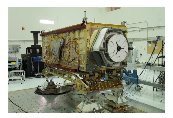
OCO-3 sits on the large vibration table (known as the "shaker") in the Environmental Test Lab at the Jet Propulsion Laboratory. Credit: NASA/JPL-Caltech NASA/JPL-Caltech
