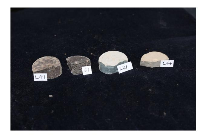
Samples of different formulations of cement that were tested for their ability to immobilize radioiodine. Credit: Canadian Light Source
