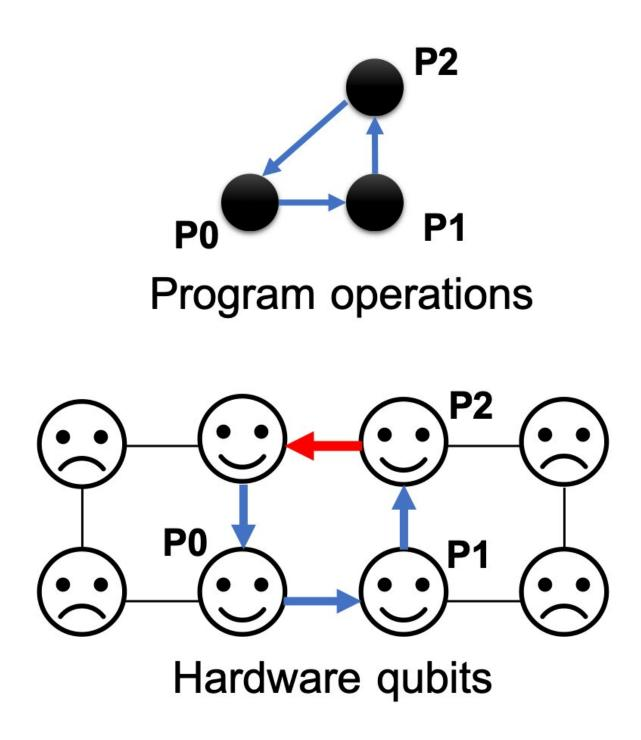
A diagram depicting the noise-adaptive compiler developed by researchers from the Enabling Practical-scale Quantum Computation collaboration and IBM. Credit: Prakash Murali/Princeton University
