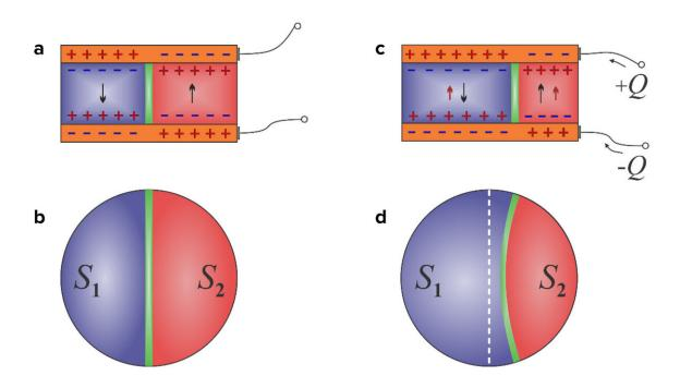
The movement of the domain wall (a-c and b-d) in a capacitor when a charge is added to one side (c). The resulting redistribution of the domain wall causes a negative capacitive effect. Credit: Argonne National Laboratory
