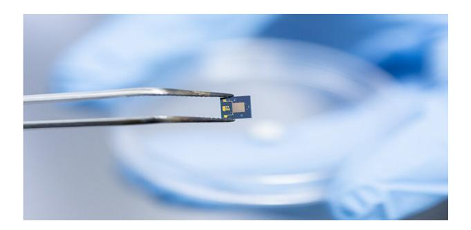
This electrode is used for collecting the sensing properties of MOFs. Credit: 2019 KAUST
