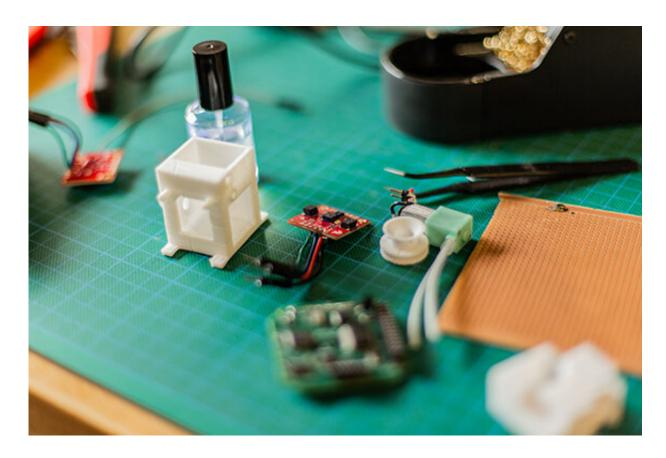
These components are important parts of the experiment. The white box is a 3D-printed chamber where the tooth and disk reside. The red electronic sensor will measure bacteria in a special broth surrounding the tooth. Credit: Swinburne University of Technology
