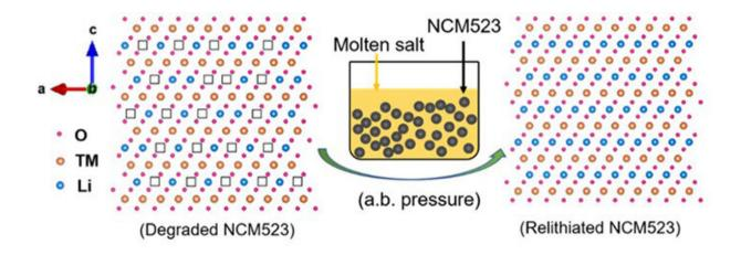
Illustration of the process to restore lithium ions to degraded NMC cathodes using eutectic molten salts at ambient pressure. Credit: Advanced Energy Materials/Chen lab
