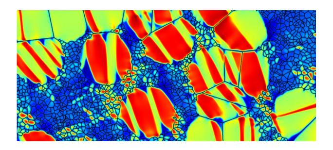
Simulated shape memory phase transition in a shape memory alloy with small and large crystal grains. Credit: IOP Publishing
