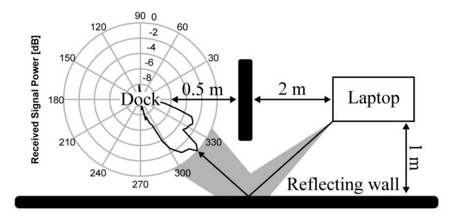
Fig. 2. Data transmission over a mm-wave channel exclusively via a reflected path. Please note that the angular energy profile does not include any lobe on the Line of Sight path Credit: © IMDEA Networks Institute
