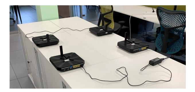
Fig. 3. Deployment of multiple consumer-grade off-the-shelf (COTS) 60 GHz access points and clients. The high directionality of the mm-wave links should limit interference, allowing multiple transmissions to take place simultaneously. However, results from TIGRE5-CM highlight that the beam patterns of COTS devices are imperfect, and side lobes may create interference. This configuration setting makes it possible to analyze the actual degree of spatial reuse. Credit: © IMDEA Networks Institute
