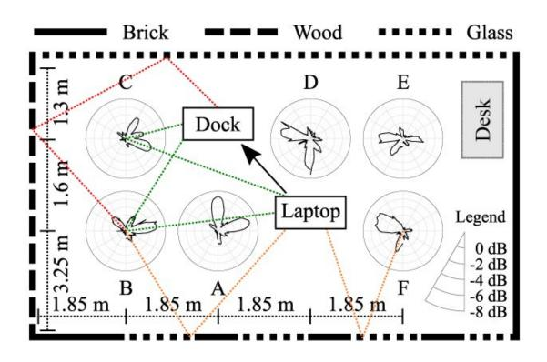
Fig. 1. Analysis of the impact of reflections patterns in a realistic mm-wave wireless setting (conference room). The dotted lines show examples of Line of Sight paths as well as first and second order reflections. The results of TIGRE5-CM highlight that these second order reflections can still be strong, hence MAC layer designs should take advantage from those to improve system performance. Credit: © IMDEA Networks Institute
