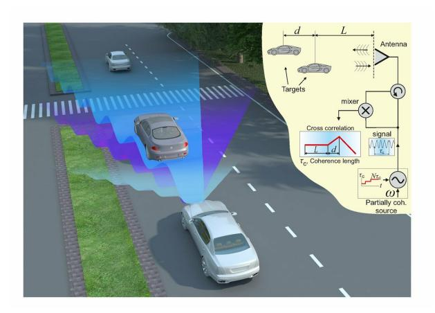
Partially coherent radar operation schematics. Credit: Nature Communications.
