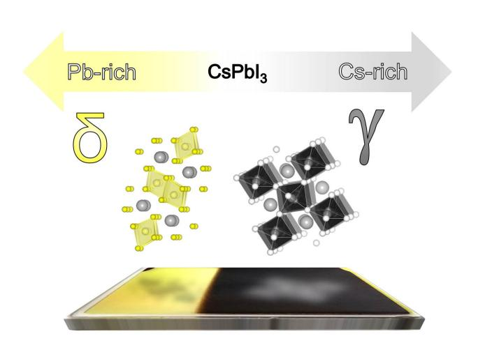
By co-evaporation of cesium iodide and lead iodide thin layers of CsPbI3 can be produced even at moderate temperatures. An excess of cesium leads to stable perovskite phases. Credit: J. Marquez-Prieto/HZB
