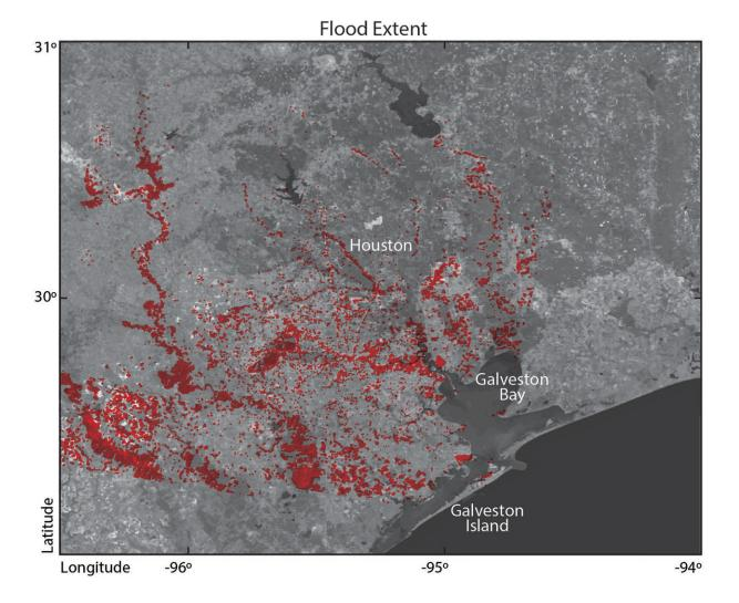
Red markers indicate inundation and standing water at 09:40 Central Daylight Time (14:40 Universal Coordinated Time) on Aug. 30, 2017, which is detected using Sentinel-1A/B SAR backscattering intensity change detection. Credit: Megan Miller
