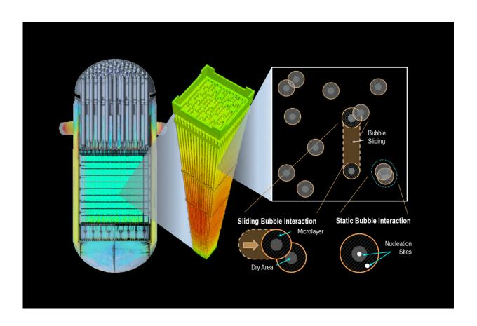
This frontal-view illustration shows the microscale mechanisms in the flow boiling framework. Each circle represents the footprint of a bubble on the heated surface, which is subdivided in a microlayer and dry area regions. Credit: Emilio Baglietto
