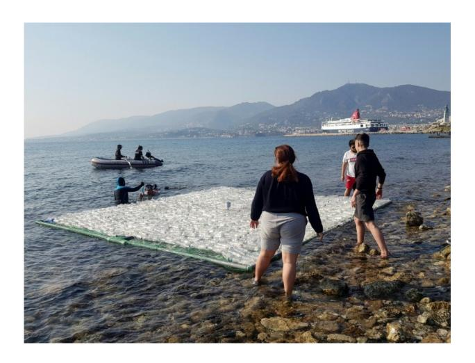
The frames are part of an experiment to determine if seaborne litter can be detected with EU satellites and drones
