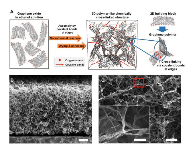
The structure of the 3DGraphene foam. (A) Schematic of the formation and structure of the bulk 3DGraphene foam. The spatial density of oxygen atoms mainly at the edges in the schematic was adjusted for clarity but did not represent its actual ratio in the material. (B) Cross-sectional scanning electron microscopy (SEM) image of the 3DGraphene foam (along the axial direction) with a homogeneous and highly porous structure. (C) Magnified SEM of the
