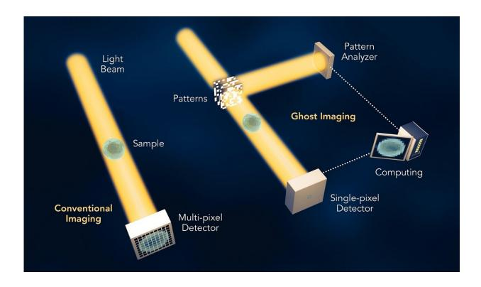
In conventional imaging (left), light falling on an object produces a twodimensional image on a detector. Ghost imaging (right) constructs an image by
