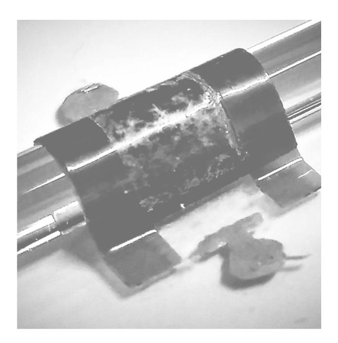
Example of a flexible and transparent electronic component: a flexible capacitor.
