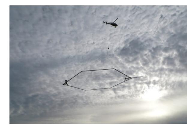
A helicopter flies over farmland near Tulare, California carrying equipment to transmit electromagnetic signals that will help gauge the structure of sand and clay layers underground. Credit: Aaron Fukuda
