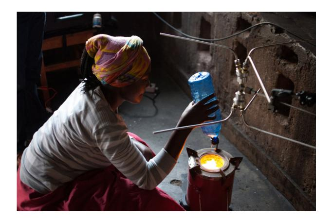
A study by North Carolina State University researchers finds that a new cookstove design, which makes use of compressed wood pellets, reduces air pollution by about 90% for a range of contaminants associated with health problems and climate change. The findings stem from a field study in which researchers worked with residents in Rwanda (as pictured here) to test the performance of the stoves in real-world conditions. Credit: Andy Grieshop, NC
