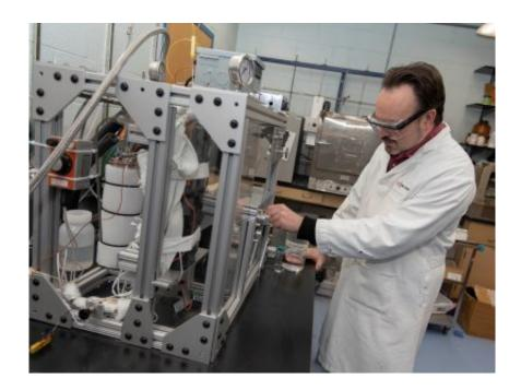
Timko inspects a high-pressure experimental apparatus that was used to measure the recovery of isobutanol into supercritical carbon dioxide. Credit: Worcester Polytechnic Institute
