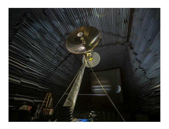
A full-scale prototype of the high-gain antenna on NASA's Europa Clipper spacecraft is undergoing testing in the Experimental Test Range at NASA's Langley Research Center in Hampton, Virginia. The Europa Clipper is expected to launch on a mission to conduct detailed reconnaissance of Jupiter's moon Europa in the 2020s. Credit: NASA/Langley
