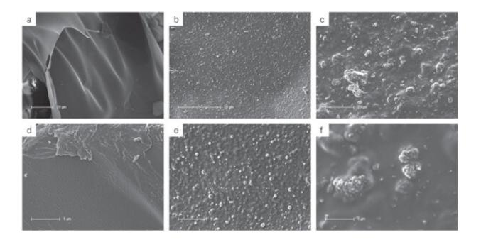
SEM images of foamed scaffolds without mineral (a), (d), with 20% ormoHAP (b), (e) or with 20% commercially available HAP (c), (f). Scale bars represent 20  $\mu$ m (top column), and 5  $\mu$ m (bottom column). Credit: Biomedical Materials, doi: 10.1088/1748-605X/ab0fad
