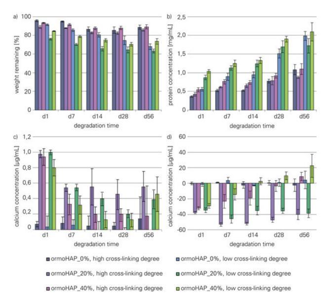
Degradation of gelatin scaffolds in PBS (a)–(c) and SBF (d) without, with 20% and with 40% ormoHAP as well as high and low cross-linking degree. Mass loss (a) and release of protein (b) as well as calcium (c), (d) in the supernatant were determined. Credit: Biomedical Materials, doi: 10.1088/1748-605X/ab0fad
