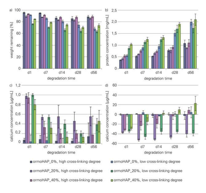
Degradation of gelatin scaffolds in PBS (a)–(c) and SBF (d) without, with 20% and with 40% ormoHAP as well as high and low cross-linking degree. Mass loss (a) and release of protein (b) as well as calcium (c), (d) in the supernatant were determined. Credit: Biomedical Materials, doi: 10.1088/1748-605X/ab0fad
