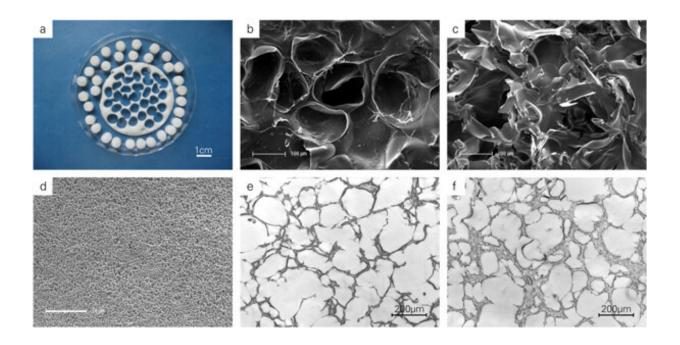
Photograph of foamed composite scaffolds used for cell culture (a). SEM images of non-foamed (b) and foamed gelatin scaffolds (c). SEM image of separated ormoHAP particles, scale bar:  $10 \mu m$  (d). Light microscopy images of semi-thin sections of gelatin scaffolds without (e) and with 40% ormoHAP (f). Credit: Biomedical Materials, doi: 10.1088/1748-605X/ab0fad
