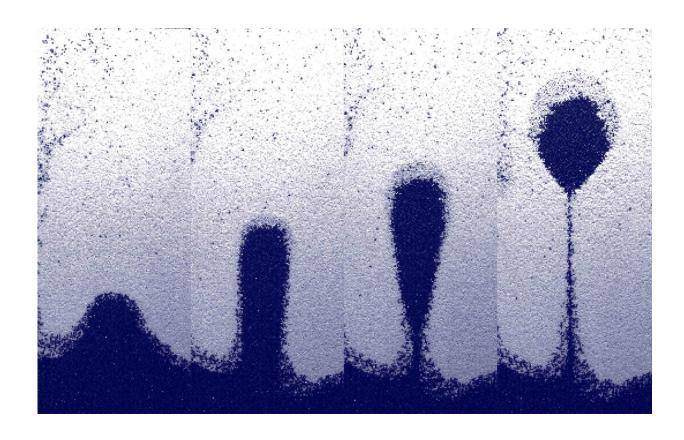
Development of a "bubble" of lighter sand (blue) forming in heavier sand (white). Credit: Alex Penn/ETH Zurich
