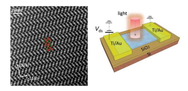
left: STEM imaging of crystal where the red and green balls represent bismuth and sulphur atoms. Right: schematic illustration of Bi2S3 detector on the Si/SiO2 substrate. Credit: ICFO
