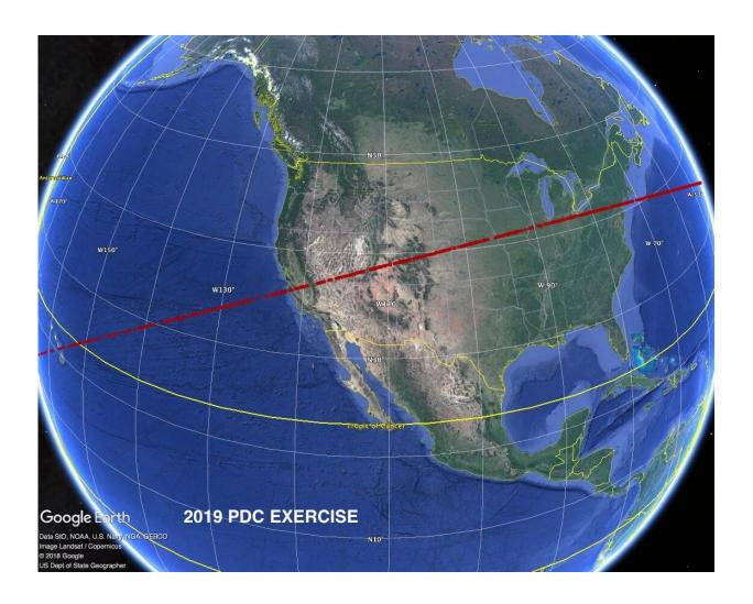
Graphic showing the hypothetical impact risk corrdior of asteroid 2019 PDC, when its orbit is still not fully known. The asteroid's uncertainty region at the time of the potential impact is much longer than the diameter of the Earth, but its width is only about 70 kilometers (45 miles). The intersection of the uncertainty region with the Earth creates a so-called "risk corridor" across the surface of the Earth. The corridor wraps more than halfway around the globe,
