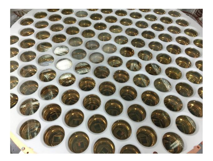
The photodetectors of the inner detecor of XENON1T were tested in liquid xenon in the UZH laboratory. Credit: Xenon Collaboration
