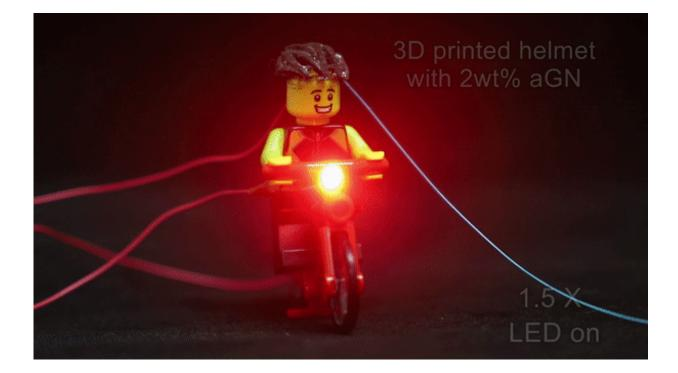
Proof-of-principle self-sensing capability of 3D printed, nacre-inspired helmet on a mini Lego bicycle rider. 3-D printed helmet with 2 wt% aGN (aligned graphene nanoplatelets), LED light is ON. Brightness decreases with crack deflection during compressive tests and resistance increases (RC circuit). When resistance increases due to crack propagation the LED turns off. Credit: Science Advances, doi: 10.1126/sciadv.aau9490
