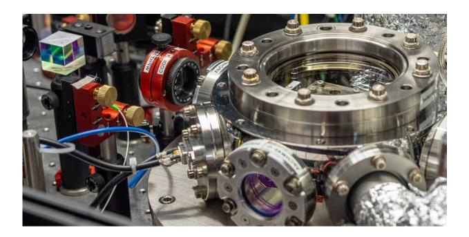
Using this sophisticated experimental set-up, the ETH researchers succeeded in cooling the nanoparticles down to a few millikelvins. Credit: S. Busschaert / ETH Zurich
