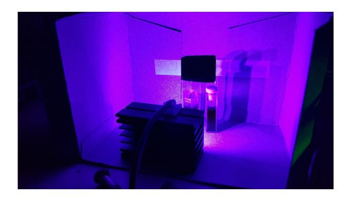
Irradiation setup to switch the photoswitchable modulator of bacterial communication from the trans-isomer to the more active cis-isomer. Credit: Dusan Kolarski, University of Groningen
