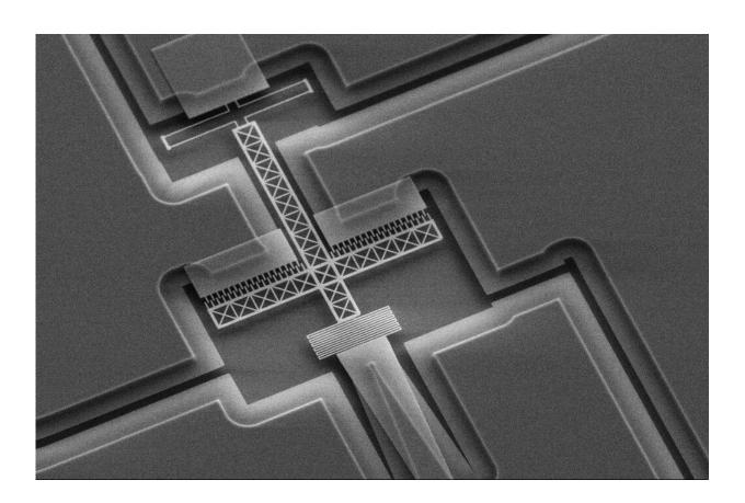
A close-up look at a miniature optical beam steering component that promises to enable lighter and less costly autonomous vehicles. Credit: Kristinn Gylfason
