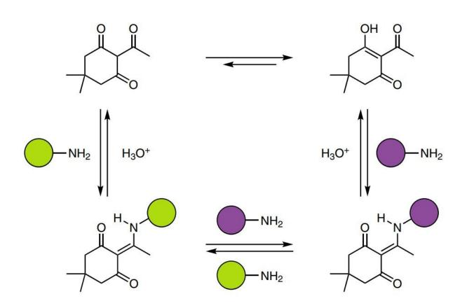
Reversible, dynamic covalent diketoenamine bonds. Diketoenamine bonds form spontaneously from triketones and both aromatic and aliphatic amines. Under strongly acidic conditions in water, the diketoenamine bond hydrolyses to the triketone and an ammonium salt. Credit: *Nature Chemistry* (2019). DOI: 10.1038/s41557-019-0249-2
