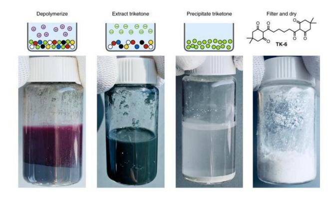
Unlike conventional plastics, the monomers of PDK plastic could be recovered and freed from any compounded additives simply by dunking the material in a highly acidic solution. Credit: Peter Christensen et al./Berkeley Lab
