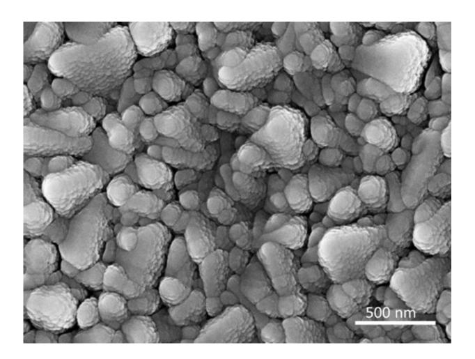
The SEM shows Molybdenum sulfide deposited at room temperature. Credit: HZB
