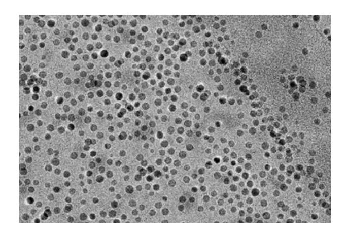
MIT researchers used these manganese oxide nanoparticles to catalyze the breakdown of water and the subsequent incorporation of oxygen into useful compounds called epoxides. Credit: researchers/MIT
