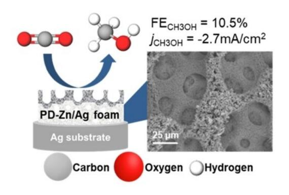
(Left) Schematic showing the production of methanol by electrocatalytic reduction of carbon dioxide using the PD-Zn/Ag foam catalyst. (Right) Scanning electron microscopy image of the surface of the PD-Zn/Ag foam catalyst. The areas with "holes" are the silver foam while the other parts show the zinc dendrites lying on it. Credit: National University of Singapore
