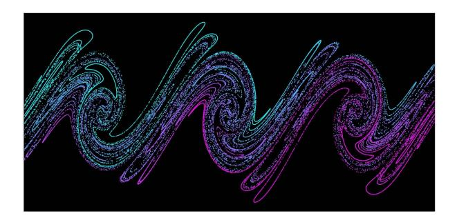
Large-scale simulations demonstrate that chaos is responsible for stochastic heating of dense plasma by intense laser energy. This image shows a snapshot of electron distribution phase space (position/momentum) from the dense plasma taken from PIC simulations, illustrating the so-called "stretching and folding" mechanism responsible for the emergence of chaos in physical systems. Credit: G. Blaclard, CEA Saclay
